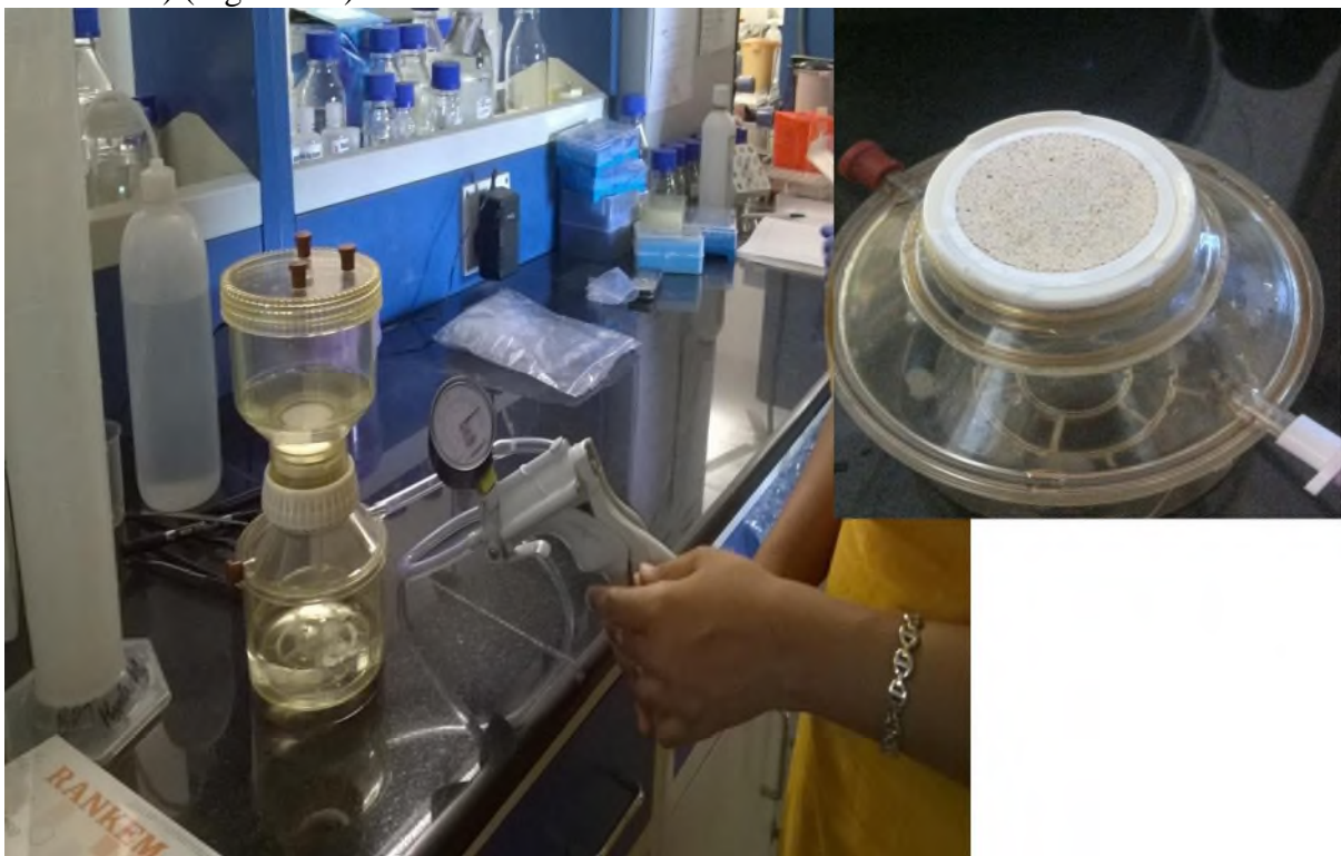
Figure 4-4: Hand held vacuum filtration unit. (Inset: cellulose nitrate membrane after filtration)
