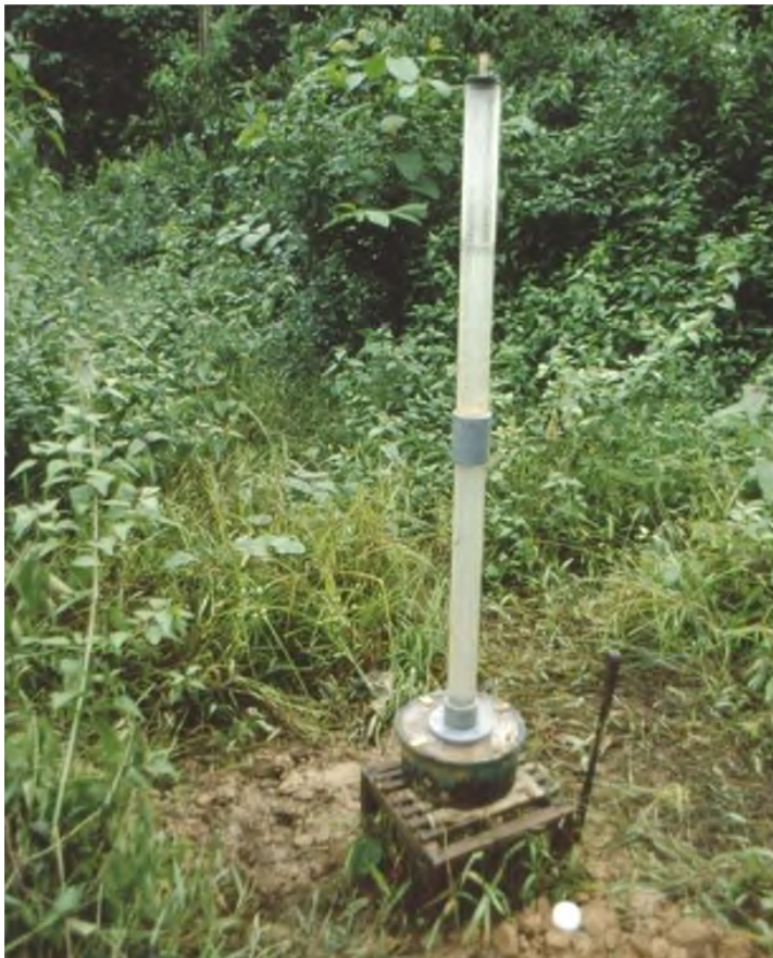
Figure 4-8: Infiltrimeter used to measure soil infiltration rates in Aghanashini
