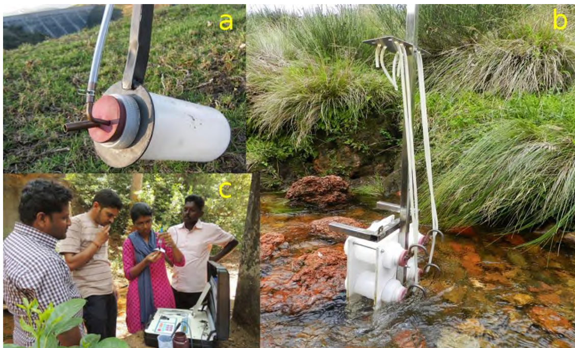
Figure 4-3: (a) Depth integrated sampler; (b) Stage sampler; (c) Demonstration of Systronics water analyzer in the field site.
