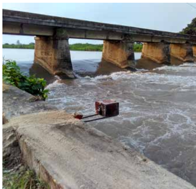
Above: Acoustic sensor installation to monitor Gandak canal level 2. © Girish Verma
